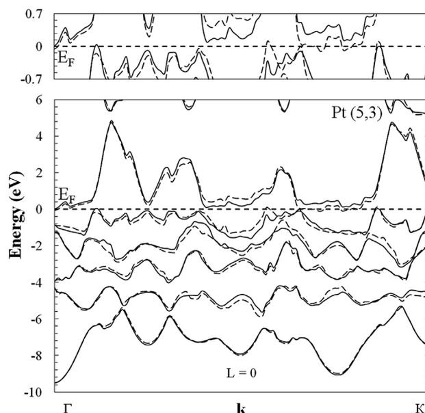
Fig. 1. Band structure of the (5, 3) Pt nanotube. The dashed and solid lines correspond to the band states with spin  $\alpha$  and  $\beta$  spins, respectively. The dispersion curves in the Fermi energy region are presented in enlarged energy scale.
