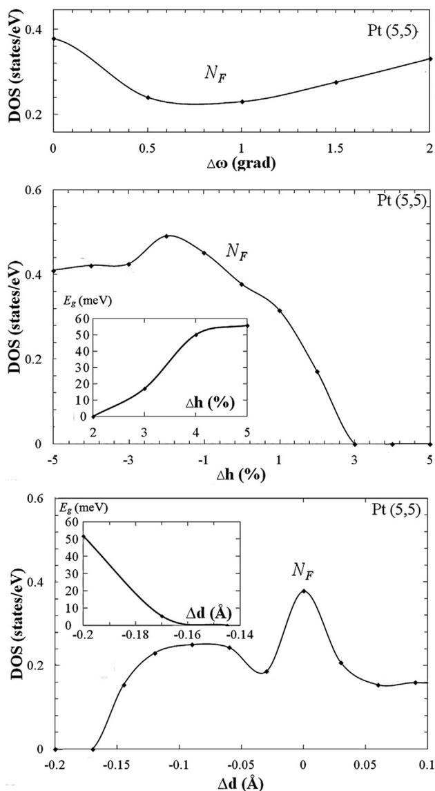
Fig. 4. Effects of deformation of (5, 5) Pt nanotube on the Fermi level DOS  $N_F$ .
