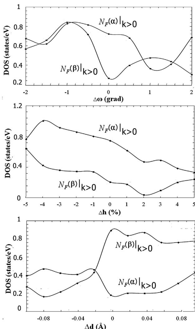
**Fig. 2.** Change of electron DOS  $N_F(\alpha)|_{k>0}$  and  $N_F(\beta)|_{k>0}$  on the Fermi level in the cases of torsional  $\Delta\omega$  and uniaxial strains, and for Pt–Pt bond variations of chiral (5, 3) Pt nanotube. Here,  $\Delta\omega > 0$  for chirality increase and  $\Delta\omega < 0$  for decrease;  $\Delta h > 0$  for tension and  $\Delta h < 0$  for compression;  $\Delta d > 0$  for stretching and  $\Delta d < 0$  for shortening.
